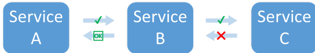
Figure 5: Service C fails when called from service B. Service B returns a degraded response to service A.
